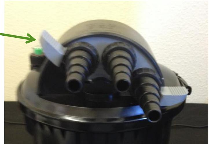
The grey handles may be a little stiff at first; do not be alarmed as this is due to the unit being new. A little bit of pressure and rocking should allow you to rotate this to change to clean mode.
