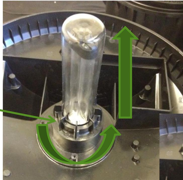
Now you are able to take out the UV bulb which is held in by pins; this will easily remove to be changed.
