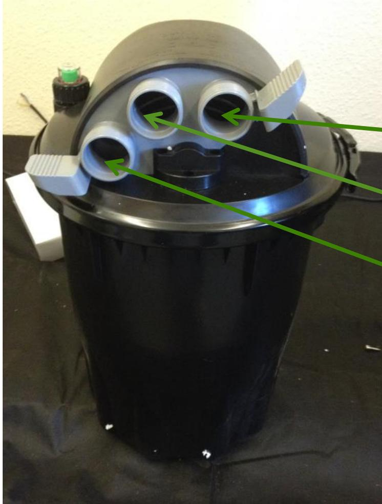
The hoesetails supplied need to be fitted securely to the screw fittings to the front of the filter unit.
