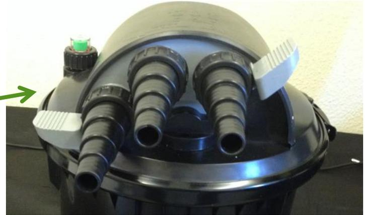
The grey handles need to be moved to the alternative position; handle down to the right to use the cleaning function.
